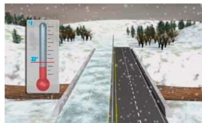
Illustration shows the road treated with SafeLane® on the left is clear after light snow accumulation
